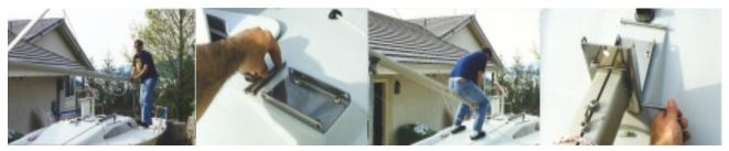
Figure 15 Walking the mast forward
