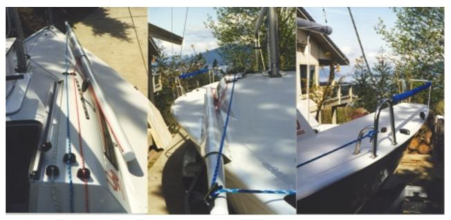
Figure 39 Spinnaker line details: halyard(next to companionway), tack line (blue) and bowsprit (red)
