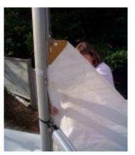
Figure 38 Feeding main luff bolt rope
