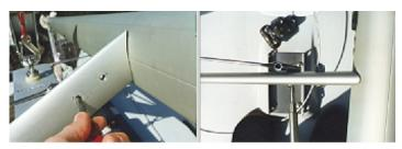
Figure 3 Lining up holes on spreader Figure 4 Tightening spreader bolts
