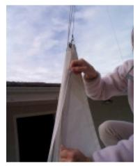
Figure 34 Zipping the luff: remember, the wire halyard and the rope tag line both go inside the zipped-up luff!
