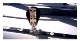
Figure 32 Jib block with standup spring in place
