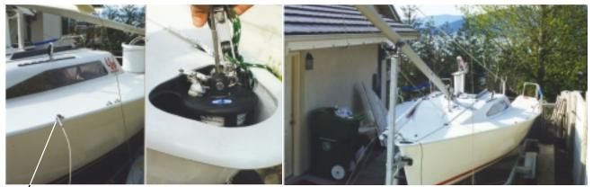
Figure 19 Lower shroud attached to forward padeye
