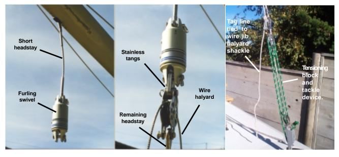
Figure 7 Short headstay hooked up to roller furling swivel
