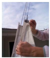
Figure 33 Jib head and zipper luff detail
