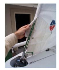
Figure 35 Green 'tensioning contraption' has been attached to the wire jib halyard
